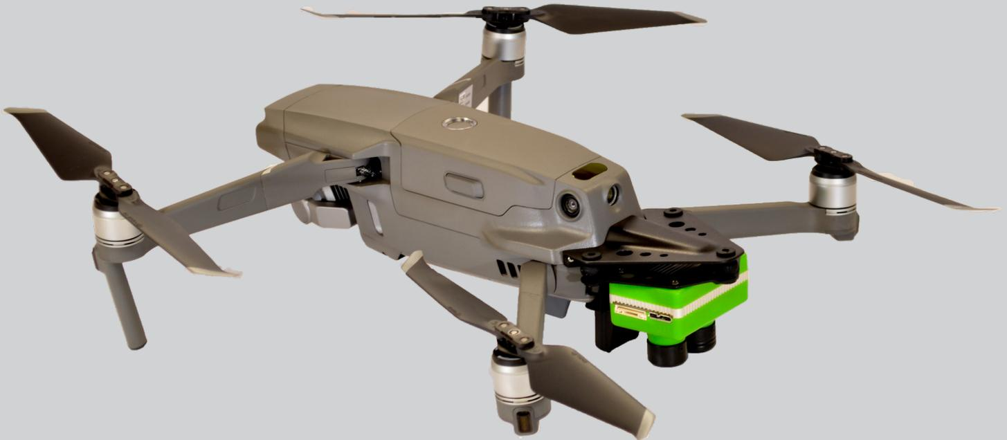
The Sentera Double 4K Sensor transforms a Mavic™ 2 Pro drone into a multi-purpose precision scouting machine. Easy-to-use, this solution allows for capture of multiple data points in a single flight, including NDVI, NDRE, and high-resolution color RGB crop health data.
