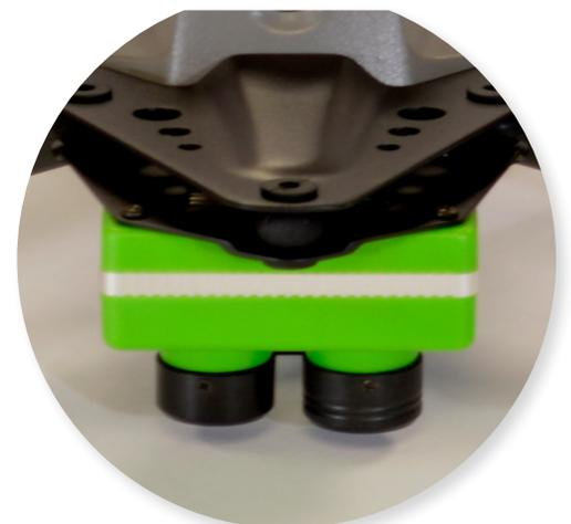
Transform a DJI Mavic 2 Pro drone into a multispectral precision scouting tool
