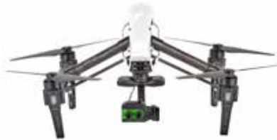
Plug-and-Play Gimbaled Double 4K Sensor on DJI Inspire 1
