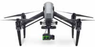
Plug-and-Play Gimbaled Double 4K Sensor on DJI Inspire 2
