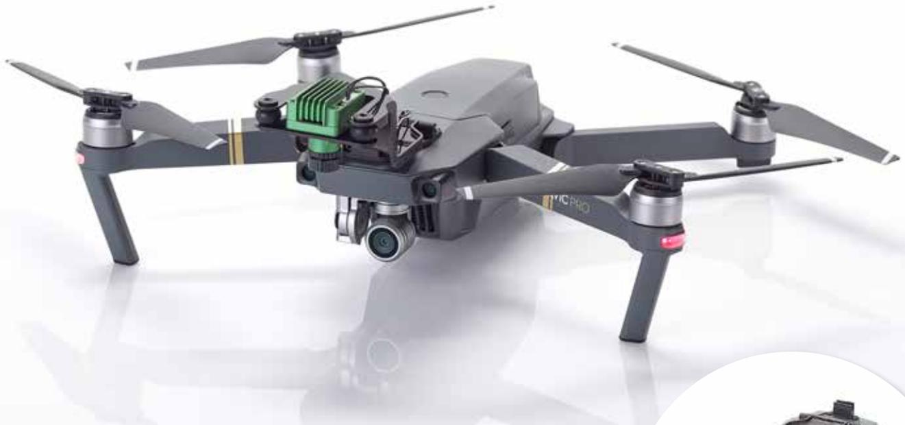
A Sentera NDVI Single Sensor transforms DJI's pocket-sized Mavic™ drone into an easy-to-use precision agriculture scouting tool. The NDVI Single Sensor enables a grower to capture NIR imagery and produce NDVI crop maps while retaining the ability to use the Mavic's 12-megapixel sensor, capable of shooting 4K video.
